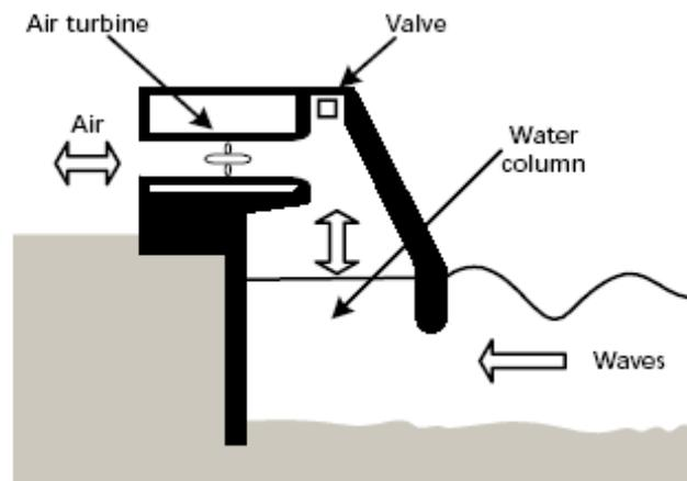
**Fig. 5 Oscillating Water Column Device [9]**
