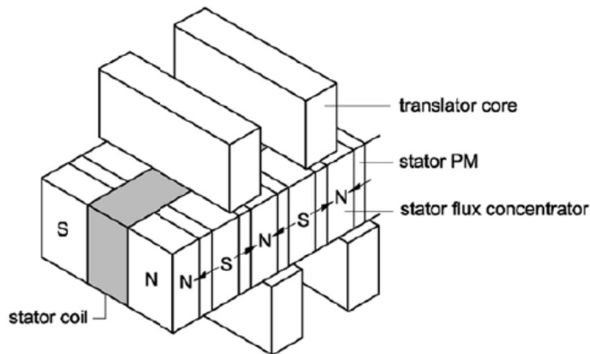
**Fig. 11 TFPM Machine with Flux Concentration and Stationary Magnets [4]**
