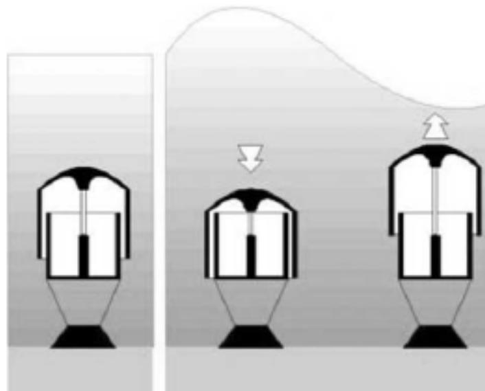
**Fig. 7 Below Surface Point Absorber [4]**
