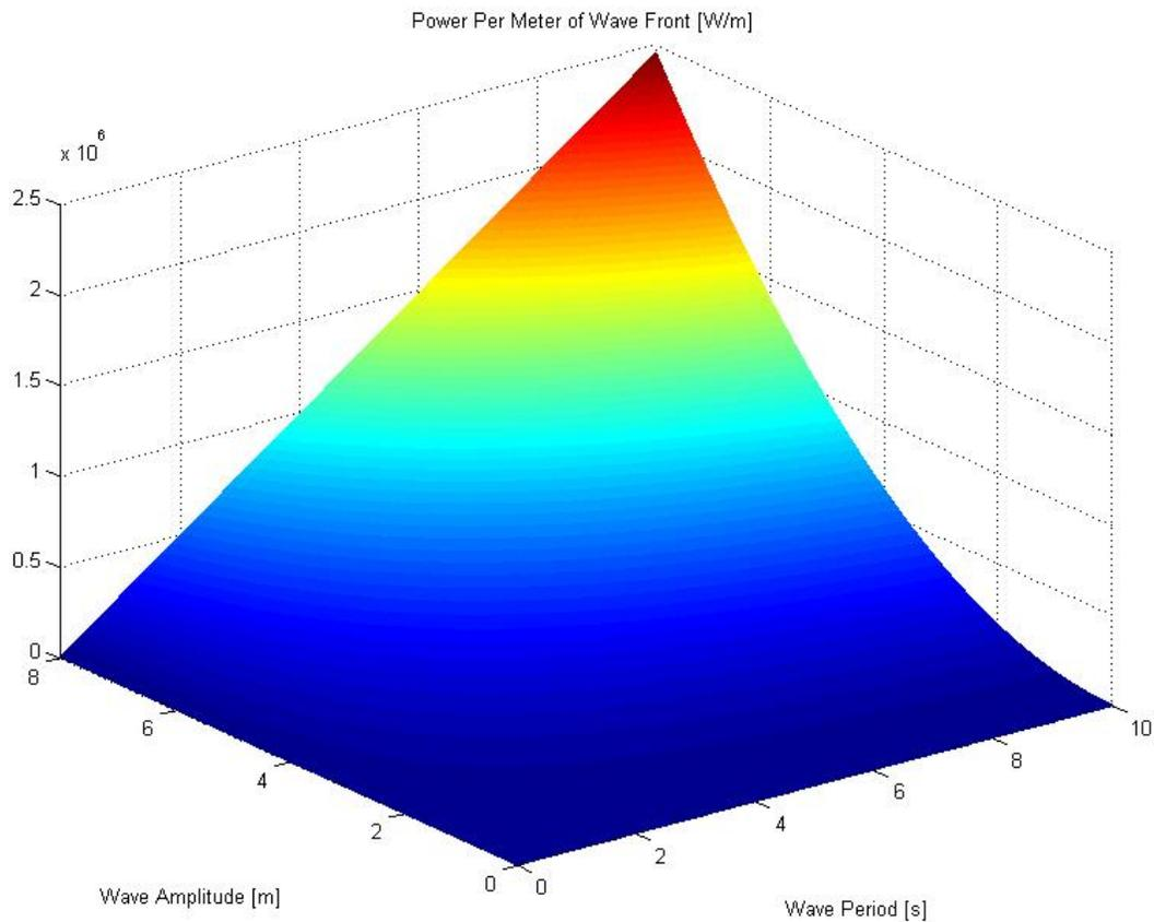
**Fig. 4 Power Per Meter of Wave Front**
