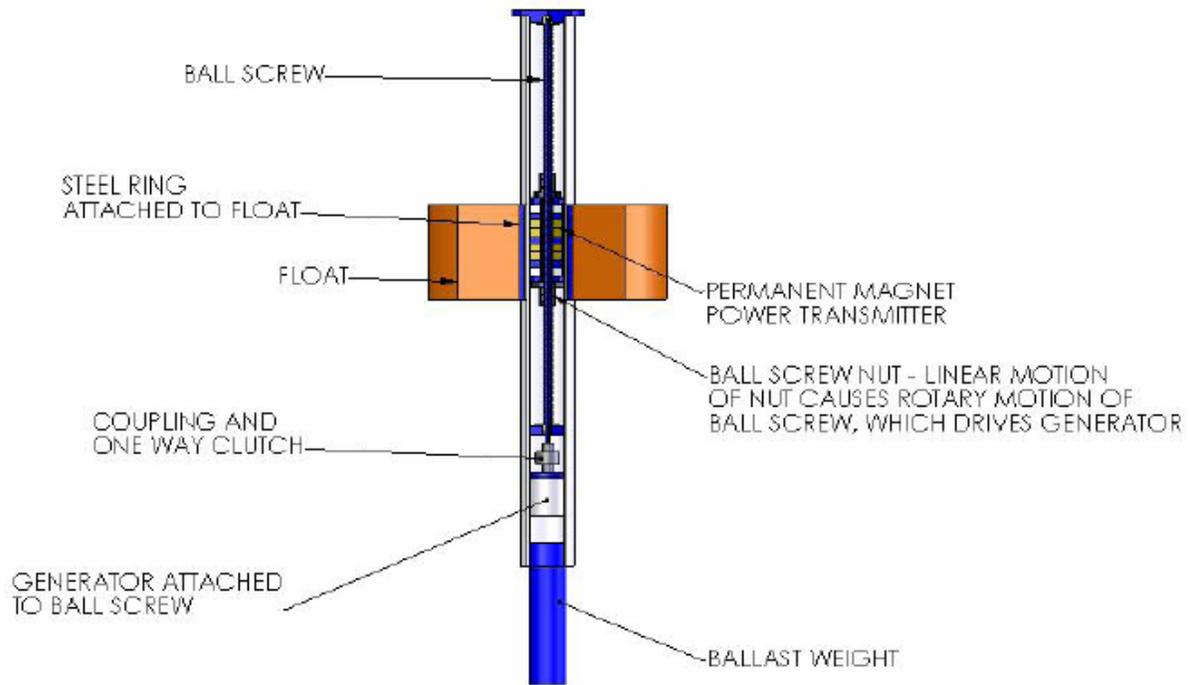
**Fig. 12 Contact-less Force Transmission System [26]**
